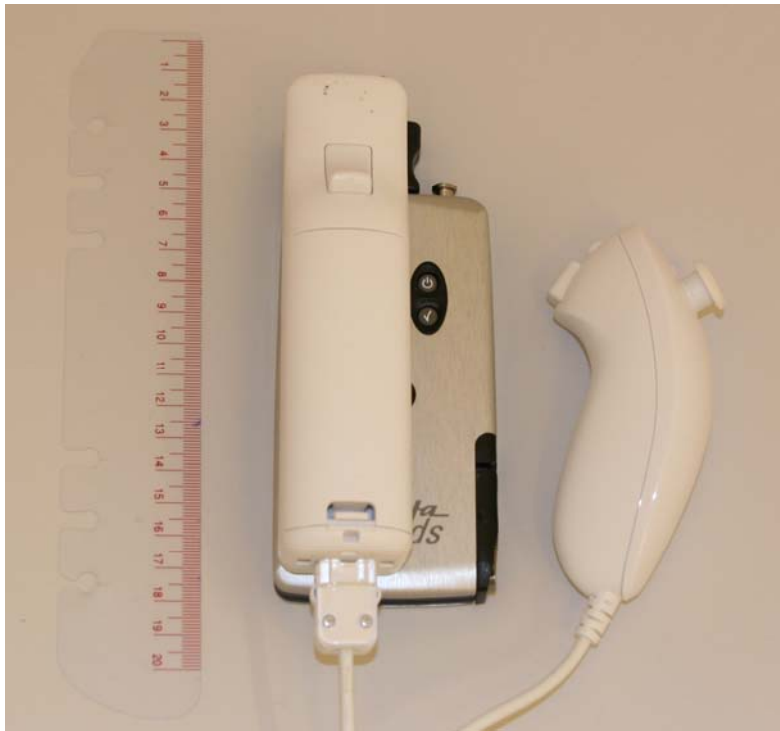
Figure 1 - White Wiimote placed on top of Embletta and attached Nunchuck (not used in this study). On left 20 cm ruler.
